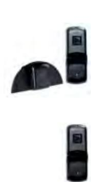
**001DBS01** Pair of wireless bidirectional infrared photocells with single contact output. Built-in receiver and external transmitter (batteries not included). For Bx-243, Bx and Bk series operators (Max range: 10 m / 32'8" ft).
