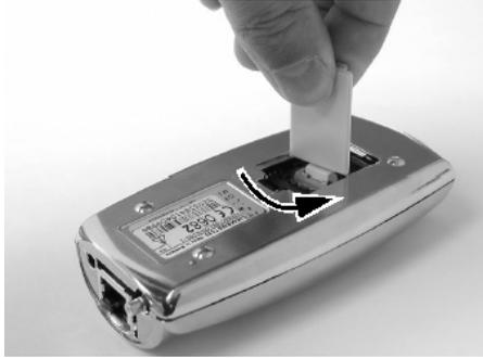
5. Flip the holder upwards. Slide the SIM card into the SIM card holder with the contact surface facing down and the flattened side at the top left:
