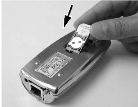
6. Press the holder down and secure it with the securing plate. Close the opening with the cover cap.
